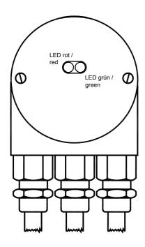
Two LEDs are implemented in the connection cap. They optically indicate the status of the encoder in the profibus network.
